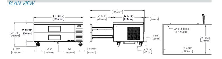
METRIC DIMENSIONS ROUNDED UP TO THE NEAREST WHOLE MILLIMETER
