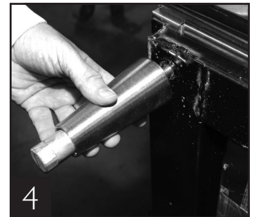
4 Thread leg into cabinet bottom frame rail.
