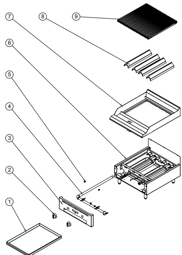
5. Remove the injectors (5) with a 1/2" wrench.
