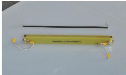
4. Remove the forcing screws from the two sides of sealing bar by Allen key, then take out the heating wire.
