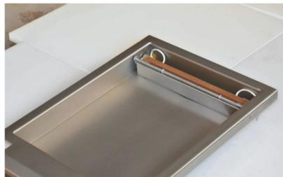
12. Connect the cable of complete sealing bar to the pin, then put the sealing bar back to vacuum chamber to finish the installation.
