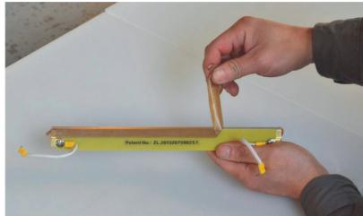
3. Pull the plastic parts out from the two sides of sealing bar by hand, then tear off the sealing tape.
