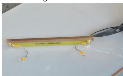
9. Cut the remaining sealing tape on the two sides enable to fold it.
