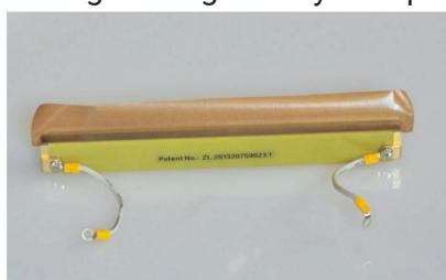
8. Take a sealing tape at proper length and sticker it on the heating wire.
