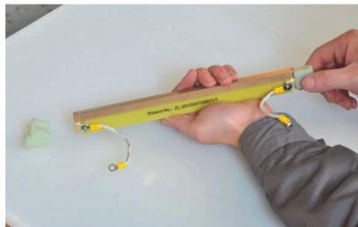
10. Put plastic parts on the two sides of sealing bar.
