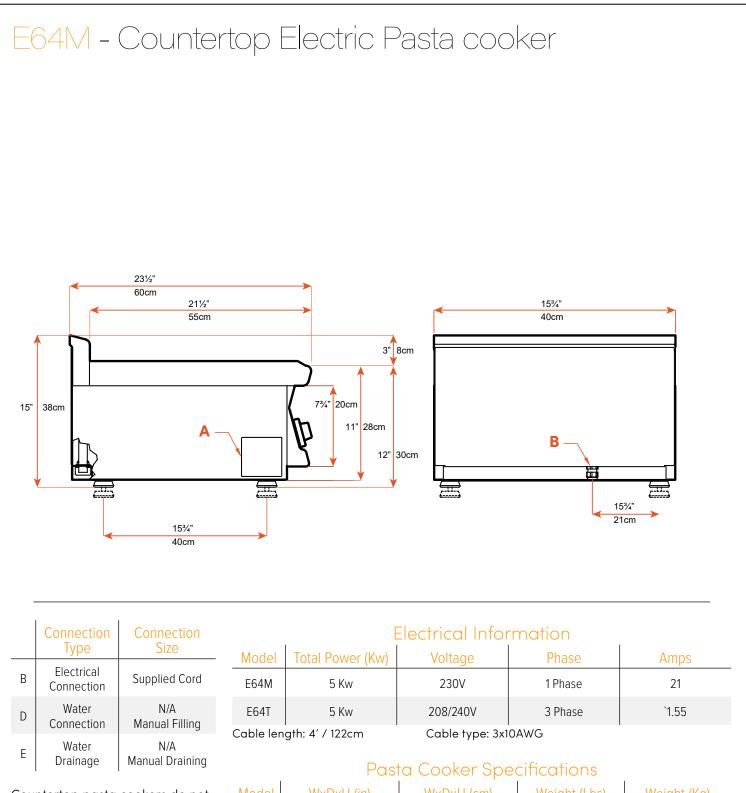
Countertop pasta cookers do not use a water connection for filling or draining. They must be filled with a hose or alternative water source, and may be drained with a spigot attached to the front drain hole.
