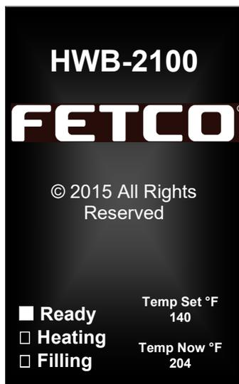
Unit has been set to ≤5° lower temperature than actual tank temperature
